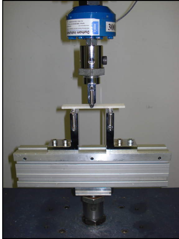
Figure 6. ASTM D790 flexural property test fixture setup. Both the loading nose and supports are fixed in their horizontal planes.
