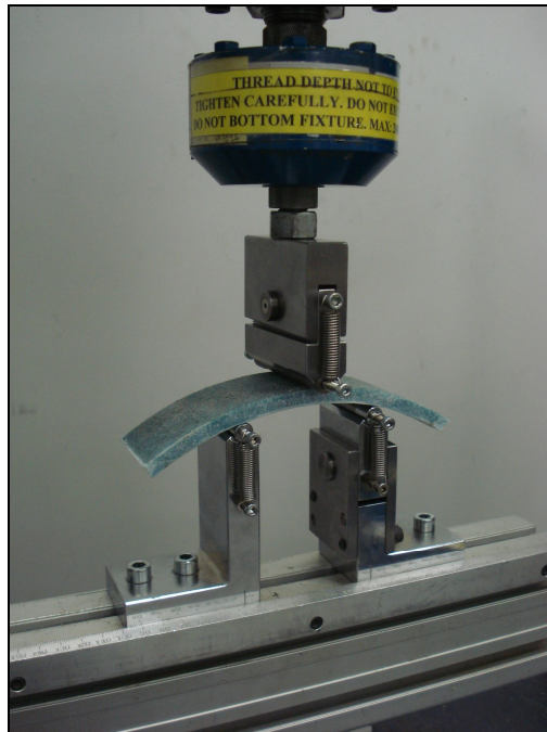
Figure 7. EN 13566/ISO 178 flexural property test fixture setup. Both the loading nose and one support are free to rotate in their horizontal planes
